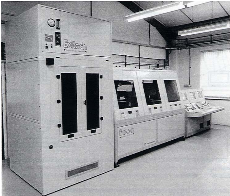
Figure 1. Exitech 193nm excimer laser microstepper system
