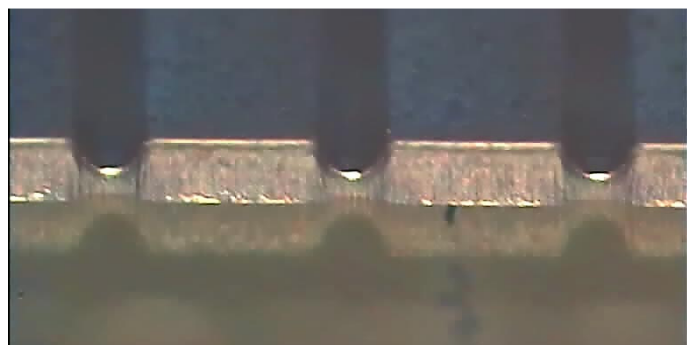
Figure 5. An array of 20µm wide semicircular cross-section fluidic channels fabricated in a dry film laminate.
