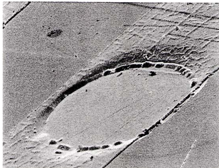
Figure 5. Electron Micrograph of a "shaped" via-hole showing the machined side to the hole where the top metal layer enters and leaves the hole. Just visible is the underlying electrode orthogonal to the top electrode.
