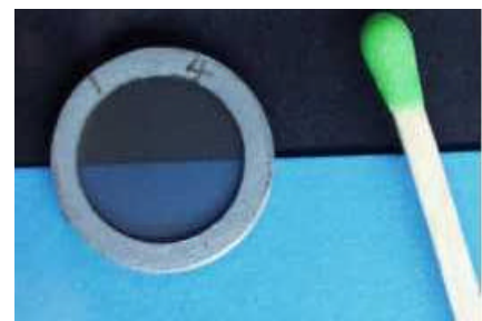
Fig. 5c: Machined Ni-dynode with 12 mm diameter
