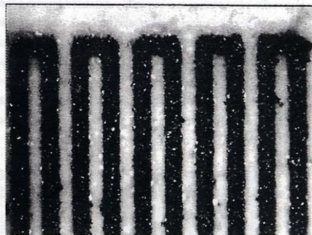
Figure 9. 25µm pitch tracks formed in screen
