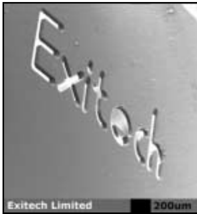
Figure 10. Direct writing using an excimer laser.
