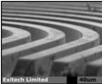
Figure 6. Curved micro-channels produced in polymer by moving the workpiece during laser firing. The shaped cross-section is determined by the mask while the sample motion defines the path of the channels.
