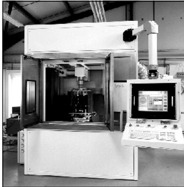
Figure 1. The Series 8000 193nm Microstepper
