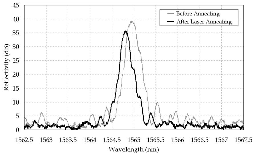
Fig.4. FBG spectra before and after laser annealing.
