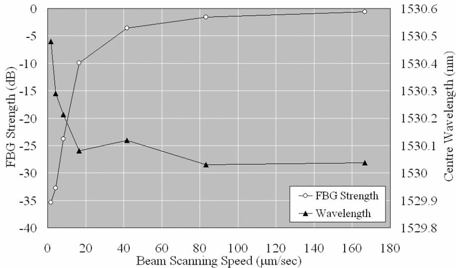
Figure 8. Variation of the strength and centre wavelength of FBGs for different beam scanning speeds from an argon ion laser.
