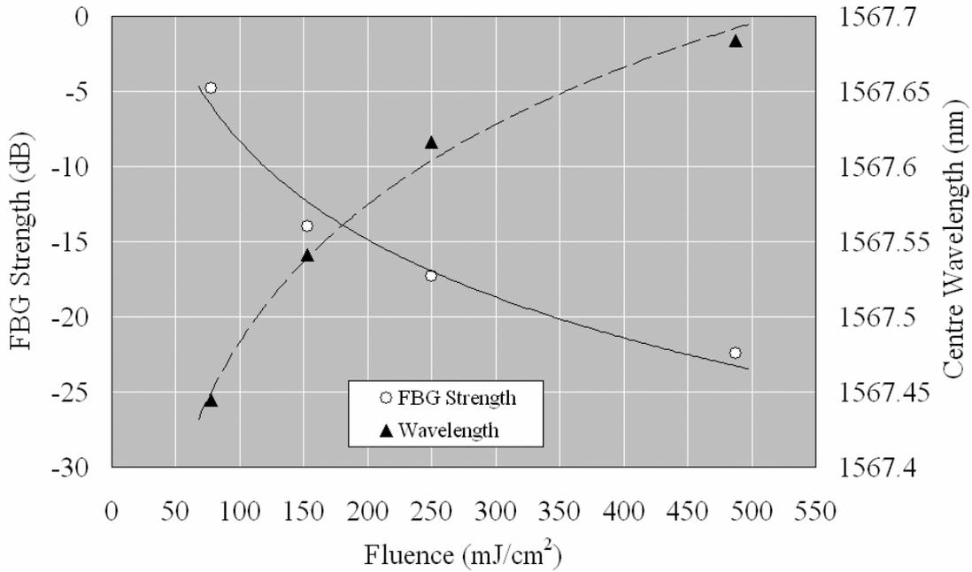
Figure 1. Graph showing variation in the strength of FBGs in H-loaded SMF28 fibres versus exposure fluence.
