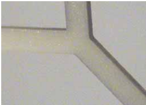
Channel layer after laser cutting
