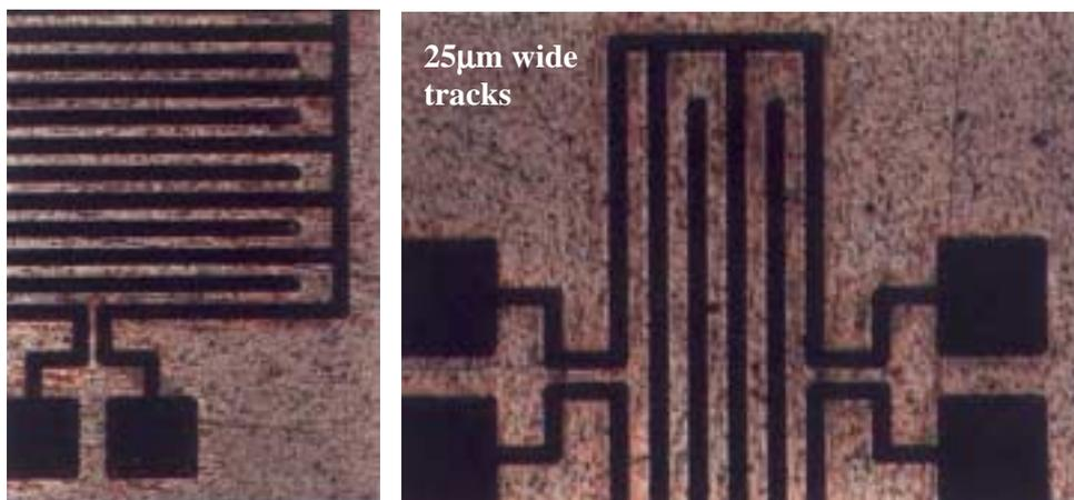
Figure 7. Circuit patterns ablated into polyimide (on copper substrate) by 3<sup>rd</sup> harmonic Nd:YAG laser.
