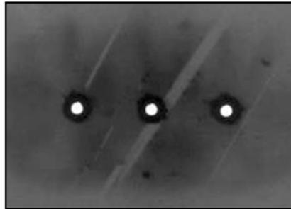
Figure 5. Inverse taper holes drilled at 355nm.
