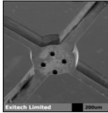
Figure 3. Nozzles machined in polyimide using multiple mask projection.
