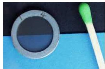
Fig. 5c: Machined Ni-dynode with 12 mm diameter
