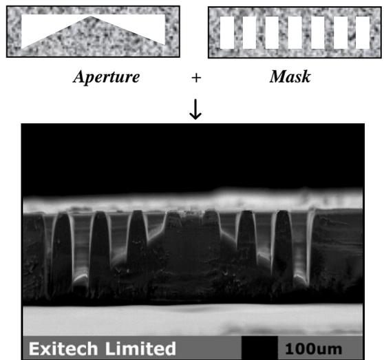
Figure 5. Micro-channels on double ramp in PET.
