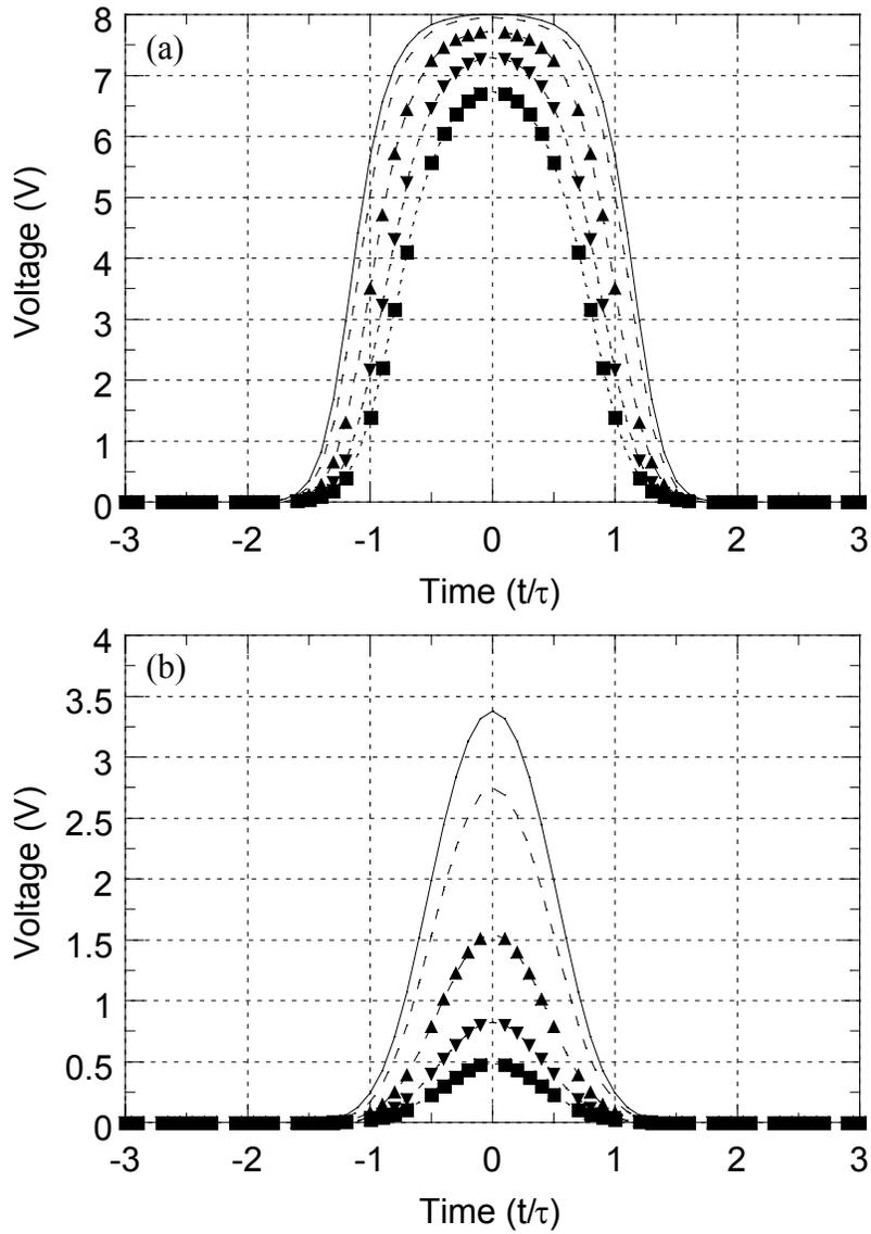
Figure 3 – Simulated response of the measurement circuit to a Gaussian pulse at 0.13 (■), 0.23 (▼), 0.48 (▲), 1.03 (dashed line) and 1.45 (solid line) mJcm<sup>-2</sup> for devices given (a) 3 treatments and (b) 7 treatments.
