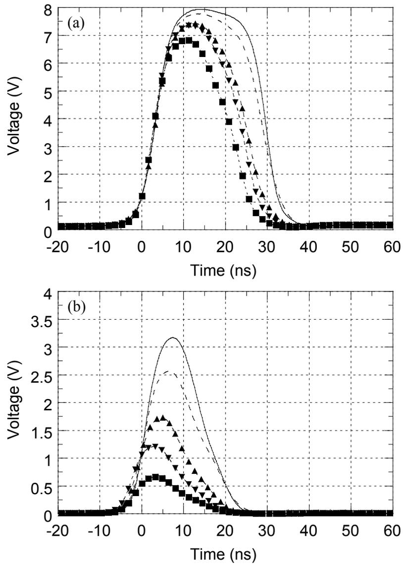
Figure 1 – Laser pulse response at 0.13 (■), 0.23 (▼), 0.48 (▲), 1.03 (dashed line) and 1.45 (solid line) mJcm<sup>-2</sup> for devices given (a) 3 treatments and (b) 7 treatments.
