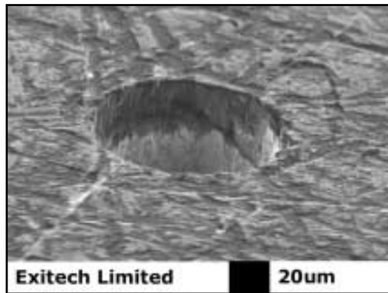
Figure 2. 100µm diameter hole drilled in stainless steel using a 355nm nanosecond pulse Nd:vanadate laser.
