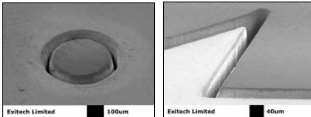
Figure 3. Glass samples micromachined using a femtosecond laser.
