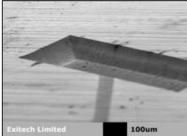
Figure 11. A microcavity machined into zirconia using a femtosecond laser.
