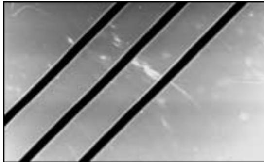
Figure 10. A chrome-on-quartz photomask where the chrome has been removed using a femtosecond laser.
