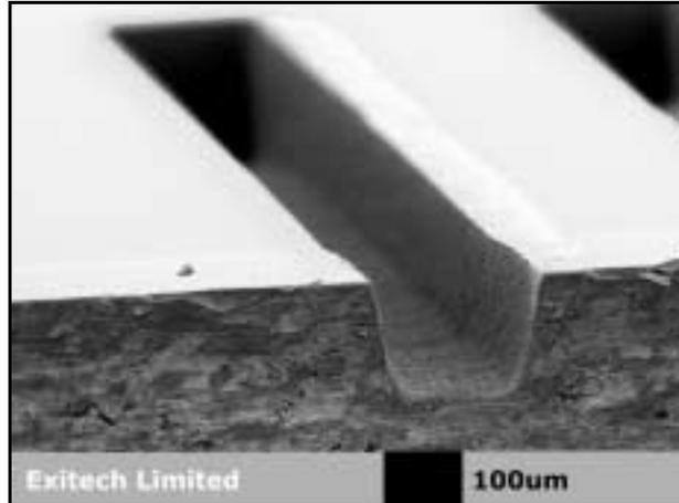
Figure 6. Trench machined into PMMA using a femtosecond laser.
