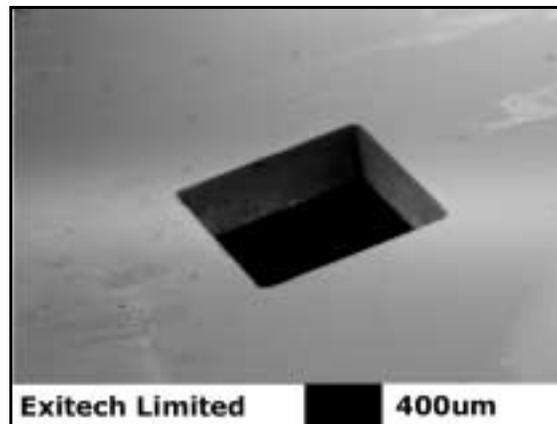
Figure 9. Sample of lithium tantalate machined with a femtosecond laser.
