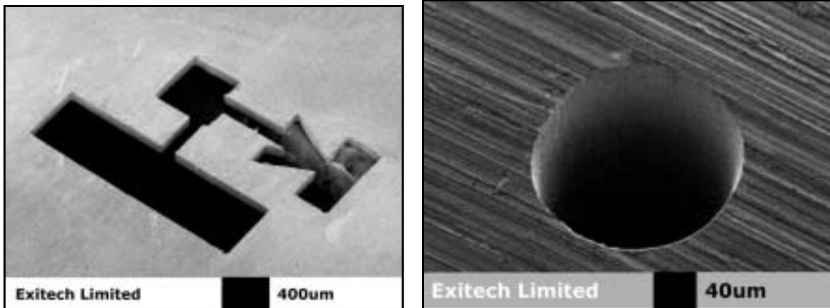
Figure 1. Femtosecond laser micromachining of aluminium (left) and steel (right).
