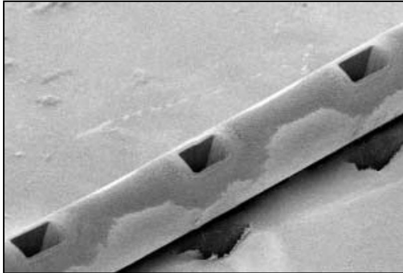
Figure 8. Direct 157nm laser micromachining of facets in silica cladding of an optical fibre.
