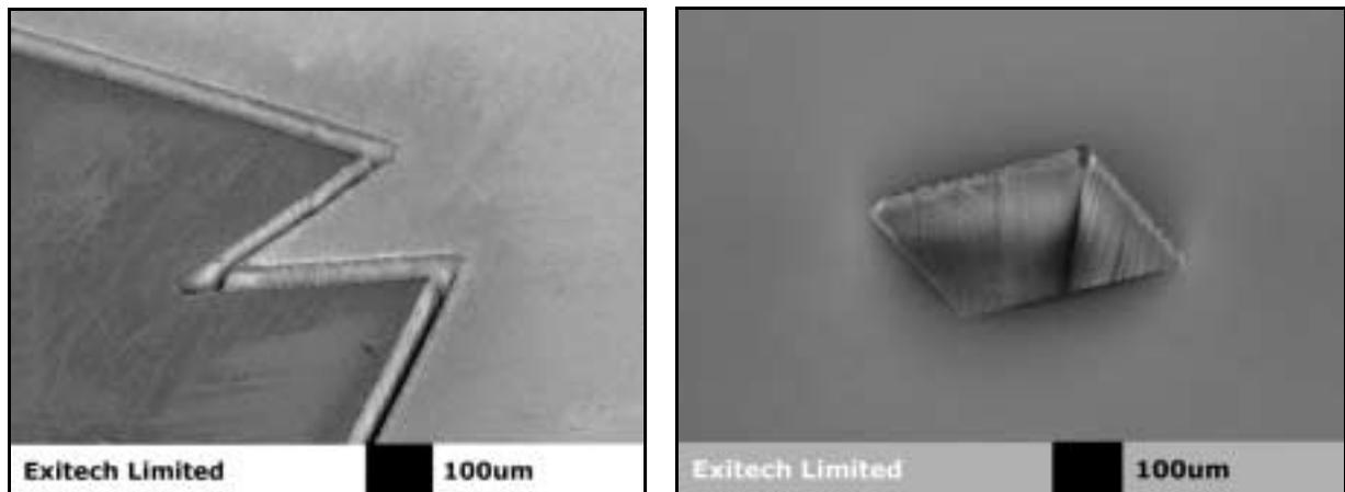
Figure 7. Samples of silica micromachined using a femtosecond laser.
