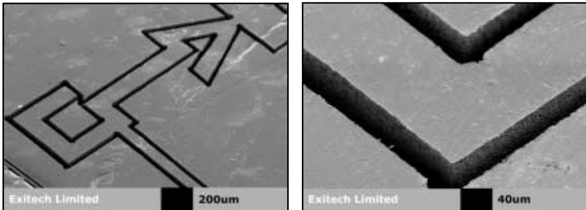
Figure 5. Samples of FEP micromachined using a femtosecond laser.
