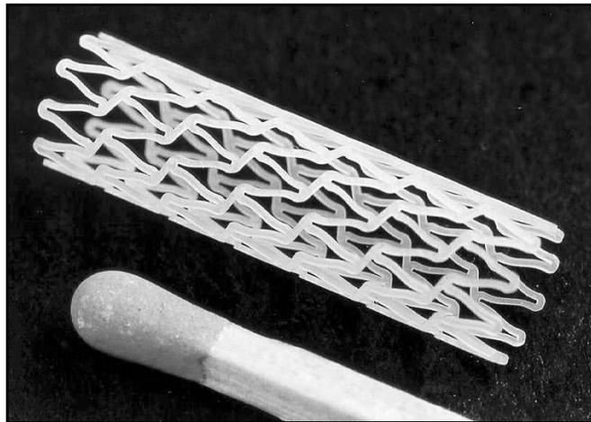
Figure 12. A medical stent micromachined from a biodegradable polymer using a femtosecond laser
