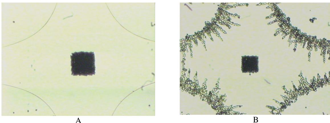
Figure 5 Developed electrokinetic microtitre wells in use. (A) The corraling of latex microbeads by negative dielectrophoresis. (B) Differential dielectrophoresis showing latex microbeads corralled by negative dielectrophoresis with simultaneous collection of yeast cells by positive dielectrophoresis.
