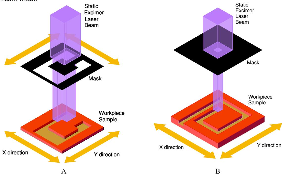
Figure 3. (A) An illustration of the principles of mask scanning laser micromachining. Mask motion is continuously synchronised with workpiece motion. (B) An illustration of direct writing excimer laser micromachining. The uniform large area beam is apertured by a static mask while the workpiece is moved. In both cases the laser beam is stationary and laser firing is triggered by incremental movement of the workpiece in either the X or Y direction.
