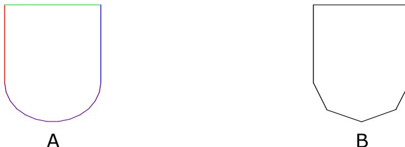
**Figure 2.** Drawing A shows a geometry made up of four different entities, three lines and a curve. Such a geometry should be presented as a single, zero-width polyline as shown in drawing B. The curve has been converted to a segmented polyline.
