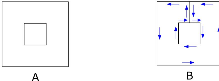
**Figure 3.** Drawing A shows an area geometry that contains a single island in the centre the area to be machined is between the outer and inner boxes. To ensure there is no confusion translating such geometries, it is better to draw them as in drawing B where the machined area is defined by a single outline which goes into the interior of the geometry and return to the edge of the geometry by the same route.
