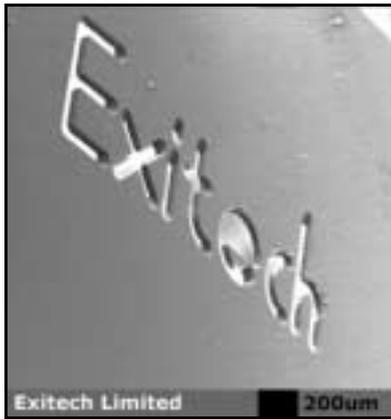
Figure 10. Direct writing using an excimer laser.
