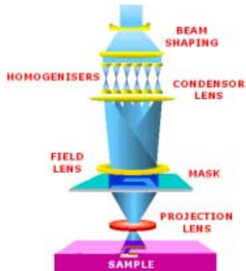
Figure 5. Schematic diagram excimer laser mask projection system.
