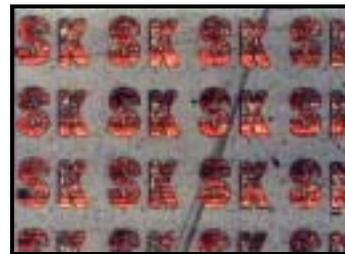
Figure 6. Polymer layer on copper selectively removed by laser ablation. The 120µm high "SK" characters are produced by step-and-repeat processing.
