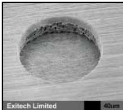
Figure 4. Hole trepanned into top copper layer using a Nd:YAG laser. Also visible is a central polymer layer which has been machined with a CO<sub>2</sub> laser and the base copper layer which is undamaged.
